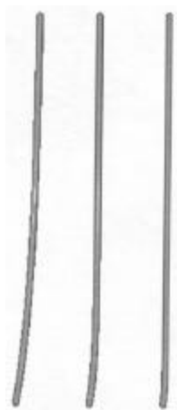
FIG. 4. Configurations of a L = 10 WLC under various stretching forces. The initial grafting angle \mu_0 = 10^\circ . From left to right: f = 0.1, 1 and 10 respectively.
