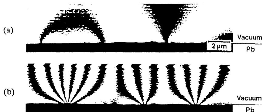
FIG. 5. Interference electron micrographs of flux lines penetrating superconducting Pb films (phase amplification: X 2). (a) Thickness = 0.2 \mu\text{m} . (b) Thickness = 1 \mu\text{m} .
