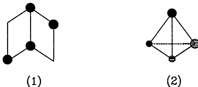
FIG. 2. Two types of chirality: (1) chiral geometry and (2) chiral substitution. Same circles denote same atoms. If the atoms were of the same species, then Type (2) would become optically inactive, although the substitution actually induces a change in interatomic distances.
