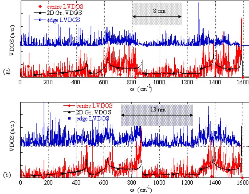
FIG. 4: Edge LVDOS (blue) and central LVDOS (red) of (a) a  $4 \text{ nm} \times 8 \text{ nm}$  GNF and (b) a  $4 \text{ nm} \times 13 \text{ nm}$  GNF superimposed on the VDOS of 2D graphene (black).
