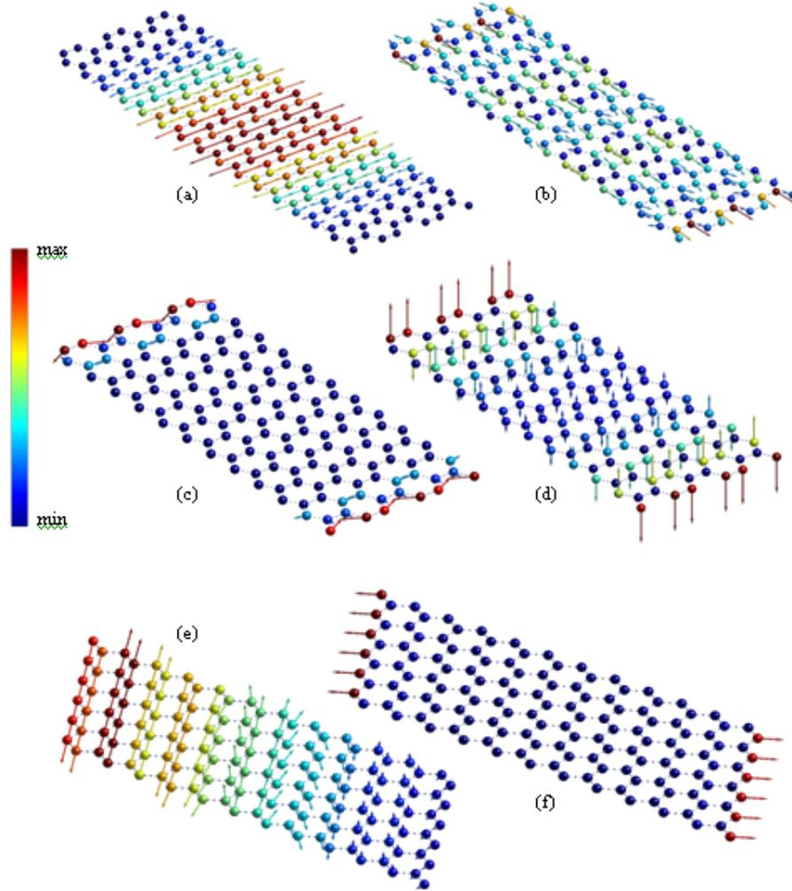
FIG. 3: Illustration of some vibration modes in GNRs: (a) Central mode in 32-AGNR at  $1460 \text{ cm}^{-1}$ ; (b) Edge mode in 32-AGNR at  $1460 \text{ cm}^{-1}$ ; (c) Edge mode in 32-AGNR at  $1350 \text{ cm}^{-1}$ ; Out-of-plane edge mode in 32-AGNR at  $630 \text{ cm}^{-1}$ ; (d,e) Edge modes in 32-ZGNR at  $480 \text{ cm}^{-1}$ .
