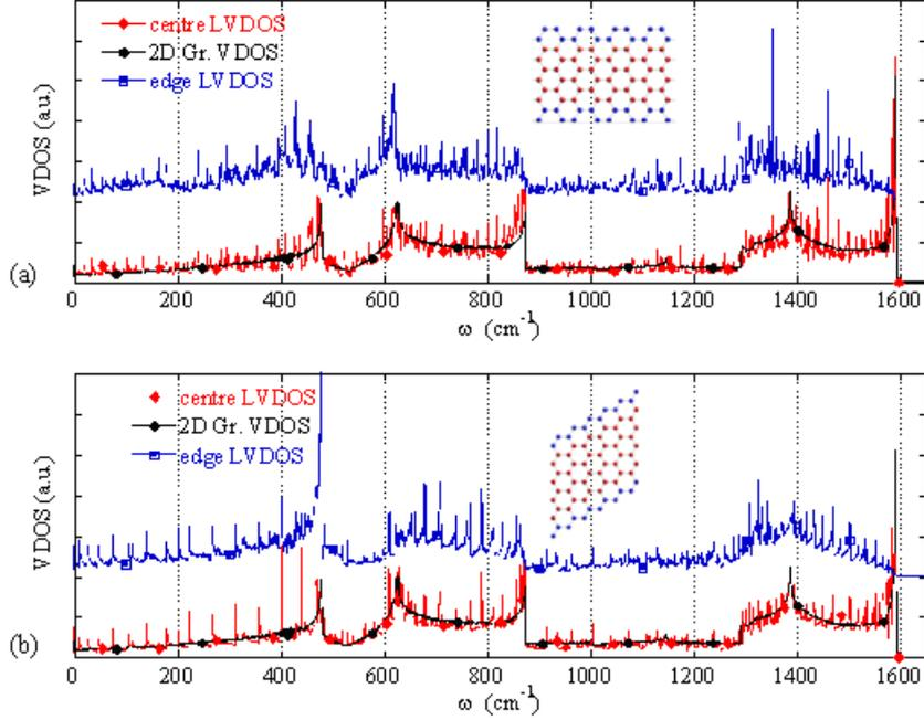
FIG. 2: Edge LVDOS (blue) and central LVDOS (red) of (a) 32-AGNR and (b) 32-ZGNR superimposed on 2D graphene VDOS (black).
