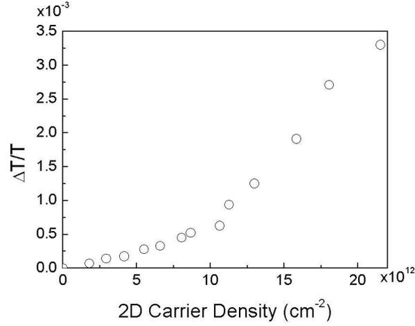
FIG. 3: Oscillation induced transmission change vs. 2D photocarrier density for the 50Å InGaN MQW sample in the single-pump pulse experiments.
