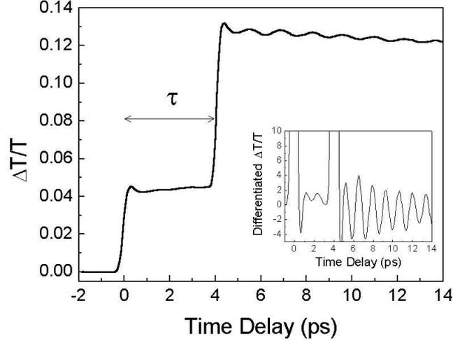
FIG. 1: Transmission change vs. probe time delay, with both pump and amplification pulses in the 50Å InGaN MQW sample. The excitation wavelength was 390 nm. The inset shows the differentiated trace, where the oscillation is more observable.
